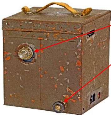
Rearview of the Beacon Crest Type A replica showing the tuning lamp P1 and the earth terminal.
